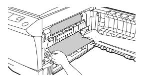
Raise the fusing unit release lever and then close the side cover by pressing the round projections near the side cover open button. The misfeed (%) indicator will go out and the ready (( ) indicator will light up.
